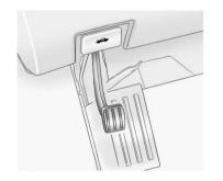
To set the parking brake, hold the regular brake pedal down, then push the parking brake pedal down.
